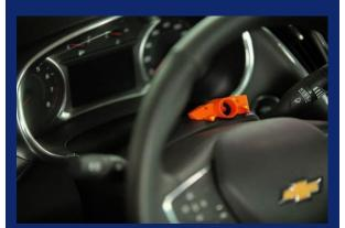
The touch system under development uses spectroscopy to measure alcohol levels under the skin's surface. A sensor shines infrared lightthrough the driver's hand or fingertip.
