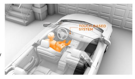
driver presses the stop/start button or wherever the sensor is located, the driver completes the loop and confirms that he or she is the person touching the button. If anyone not in the driver seat presses the button, the circuit will not be closed and the alcohol measurement will not be considered valid.
