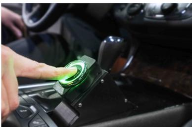
**The touch system** uses tissue spectroscopy to measure blood alcohol levels under the skin's surface by shining an infrared light into the fingertip or palm of the driver. It is being designed to take multiple, accurate readings in a matter of seconds. While final locations are still being determined, it will likely be integrated into current vehicle controls, such as the gear shift, starter button or steering wheel.
